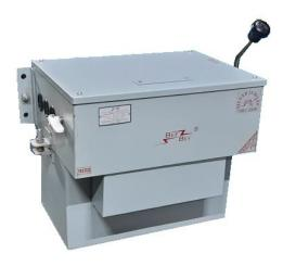
NSD is manually operated, oil immersed wall mounting type, Star/Delta Starter suitable for 415 VAC 3 Phase, 50 Cycles, A.C. supply, without first filling of oil, Ammeter and unpacked as per IS: 8544 (Part-I1)-1977.
